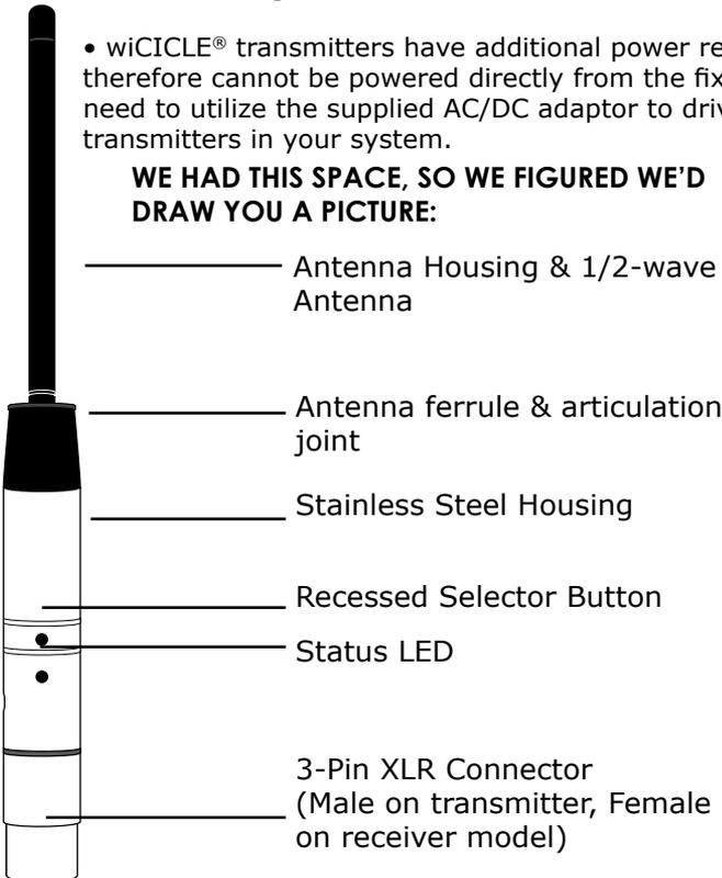
Each wiCICLE® acts as both a transmitter and a receiver, depending on whether a DMX source is applied to the integral XLR connector. This is an extremely powerful feature of the system, however, it also requires 1 piece of due diligence, and that is the removal of extraneous DMX signals from your lighting rig BEFORE proceeding.
